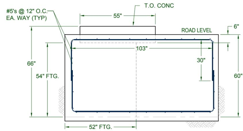
**REINFORCEMENT SECTION "A-A"**
