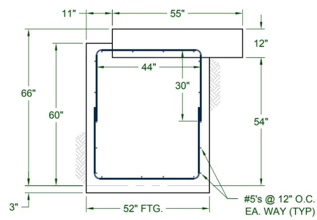
**REINFORCEMENT SECTION "C-C"**
