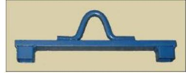
The lifting bar is secured to the top of the slide tube by two bolts. A sling can then be passed through the ring so that the weight can be supported by suitable lifting equipment.
