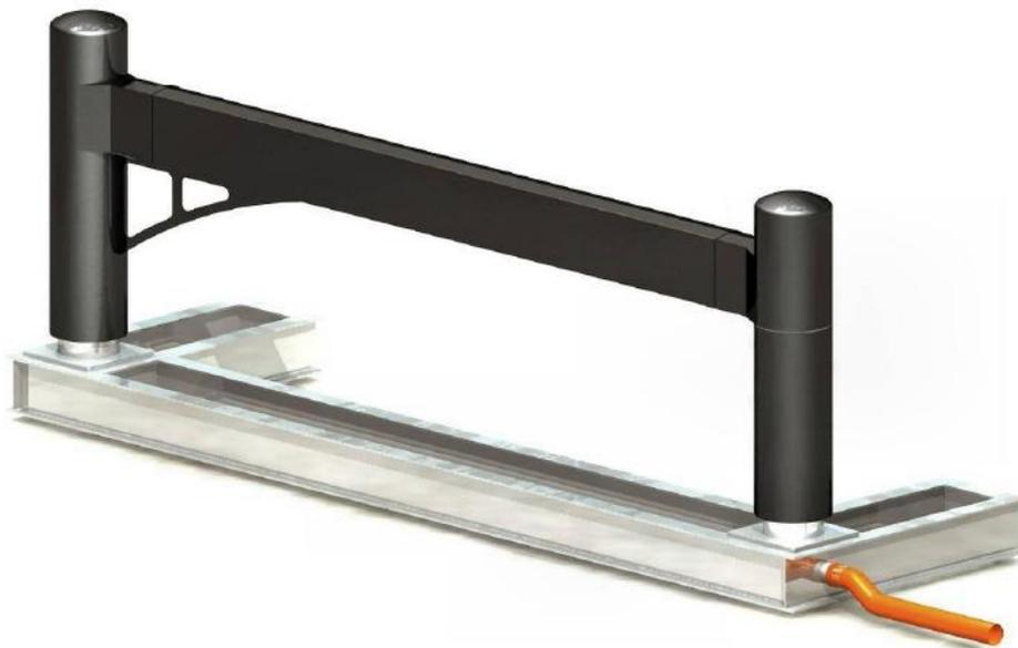
The hydraulically driven locking pin is housed in the right hand end of the gate in the above illustration and is driven vertically up and down by a hydraulic ram. If required, the hydraulic power pack and electrical controls needed to operate the ram, to unlock and lock the gate, are housed in a remote control panel which requires a 208/1/60 electrical supply.
