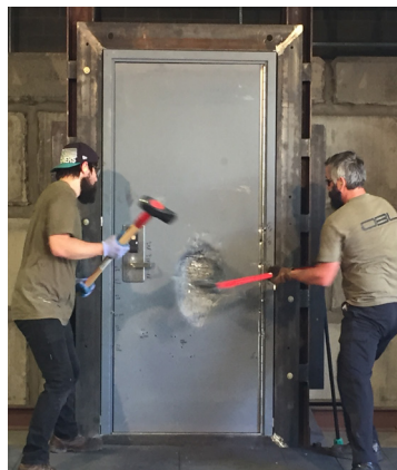
Image from actual forced entry testing
